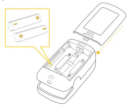
Install batteries with the positive (+) and negative (-) terminals properly aligned with the corresponding symbols in the battery compartment
